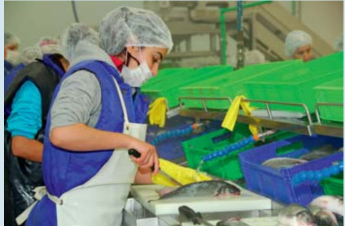
Sophisticated equipment is used for most processing operations, but the filleting is all done by hand as it results in higher yields.
