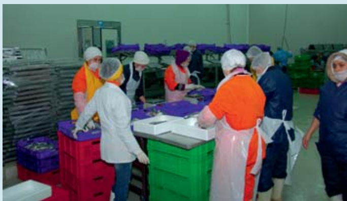
The fillets are weighed and packed in styrofoam boxes on ice.
