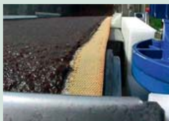
Figure 6.2 Hydrotech belt filter used for dewatering the sludge. Source: Hydrotech.
