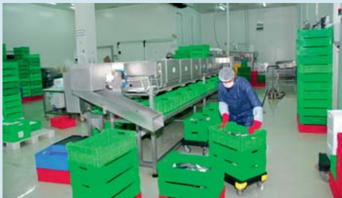
Seabass and seabream is automatically graded before being sent for further processing.
