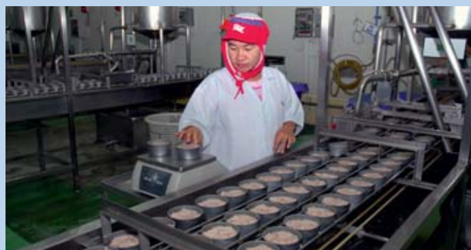
Random samples are taken before the cans are sealed to check that the fish weight meets the specifications.
