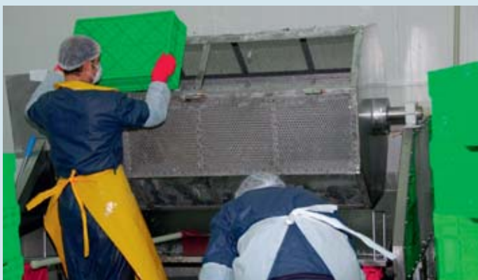
The fish is descaled by rotating it in a machine that rubs the scales off.
